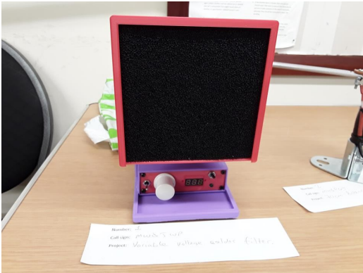
Above: Solder Station Filter, using 3D printed parts, by John MW0JWP
