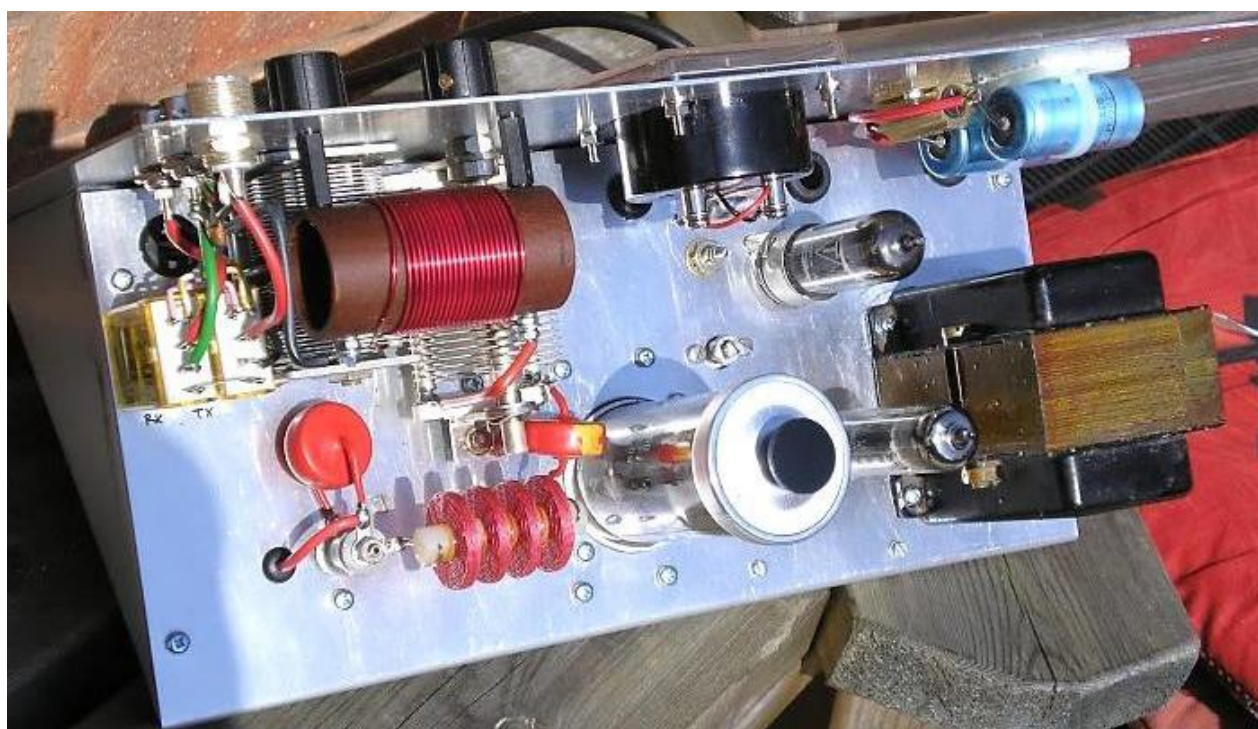
Figure 10. Top-side of the RF deck with the modulation transformer on the right hand side
