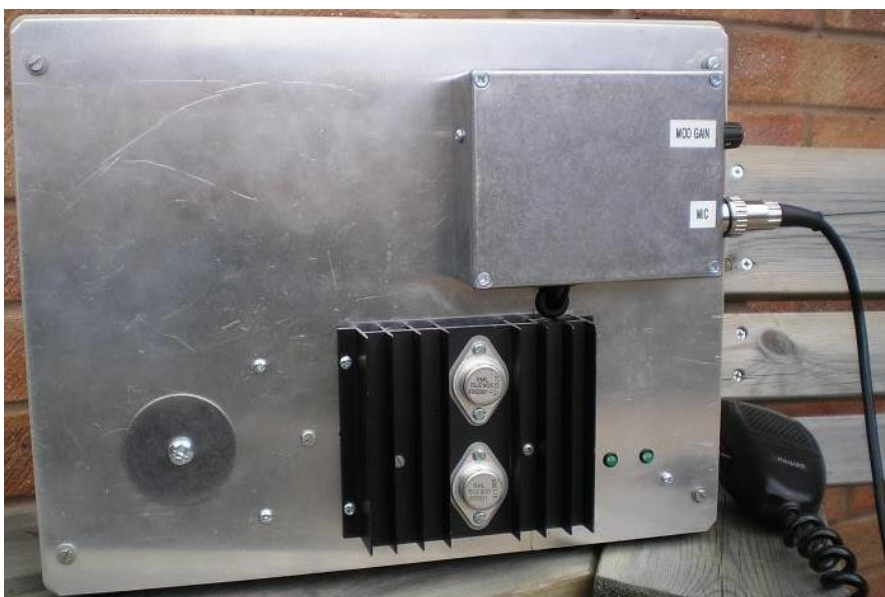
Figure 8. The heatsinks for the MOSFETs are mounted on the outside of the rear panel, together with the speech processor in a die-cast box
