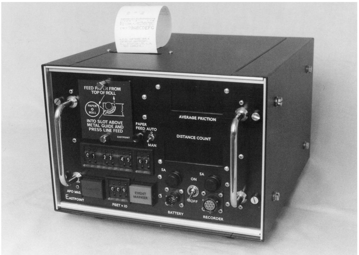
The electronics unit for the Mu Meter. Note the legend 'Eastpoint' at bottom left, which was our company name.
