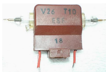
Figure 1. Reed switch used to switch the HV supply
